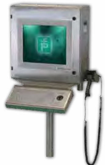
Div. 1 Operator Workstation with intrinsically safe keyboard and barcode reader
