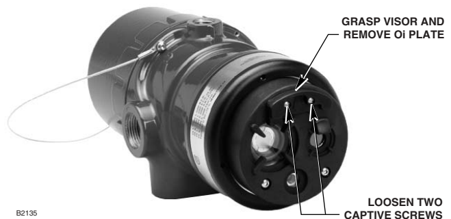
Figure 17—Oi Plate Removal
